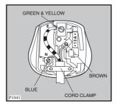
The wire coloured green and yellow must be connected to the terminal marked with the letter  $\langle E \rangle$  or by the earth symbol  $\frac{1}{2}$  or coloured green and yellow.
